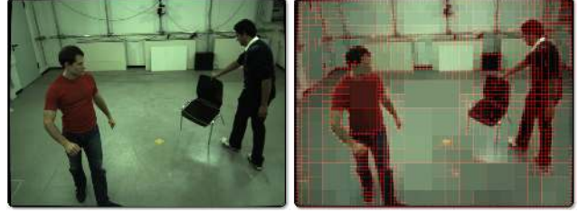
Figure 2. SoG image approximation. Left: Input image. Right: Quad-tree structure with average colors used to generate the SoG. Each square is represented by a single Gaussian.
