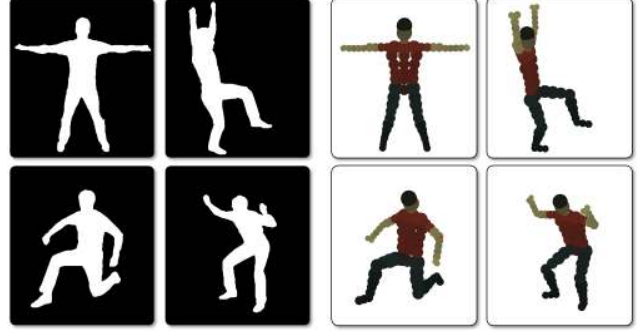
Figure 5. Estimating an actor specific model from example pose images. Left: Single segmented input image of the multi-view sets for each pose. Right: Resulting actor-specific body model after optimization and color estimation.
