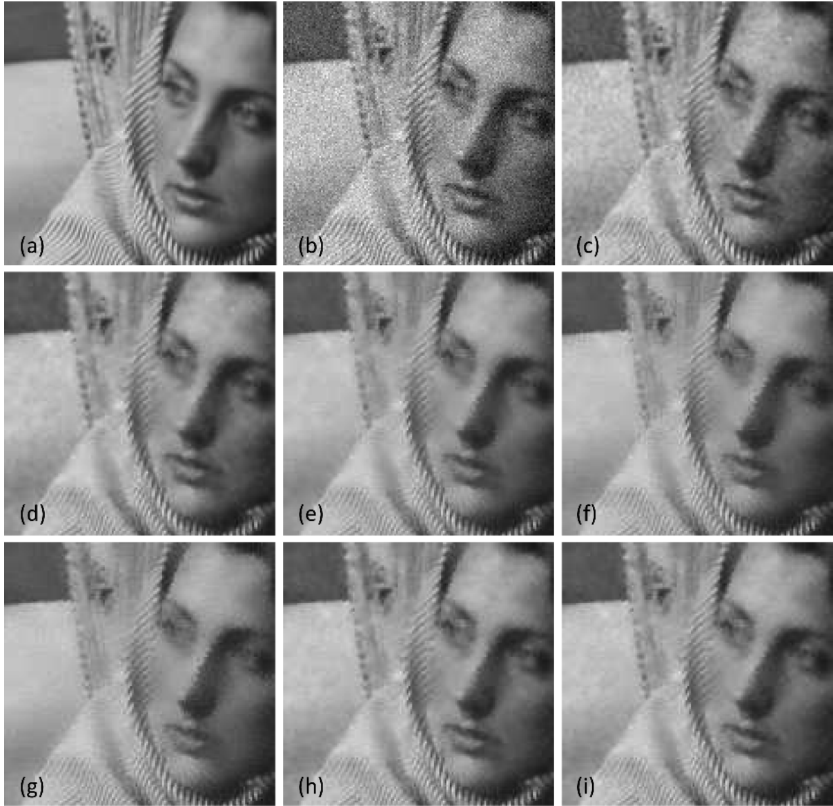
Fig. 4. Denoising example. (a) Input image. (b) Noisy image with noise standard deviation of 15 (PSNR = 24.64 dB). (c) Box bilateral filter with N = 1 (PSNR = 28.44). (d) Box bilateral filter with N = 2 (PSNR = 28.56). (e) Box bilateral filter with N = 3 (PSNR = 28.55). (f) Box bilateral filter with N = 4 (PSNR = 28.42). (g) Box bilateral filter with N = 5 (PSNR = 28.22). (h) Standard bilateral filter (PSNR = 28.84). (i) Proposed bilateral filter with M = 5 (PSNR = 28.73). The quantization level is 15, \sigma_r = 30 , and \sigma_d = 1.8 .
