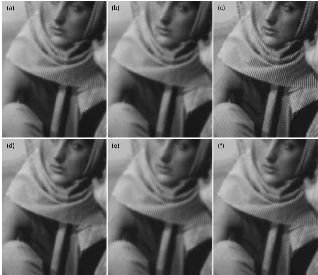
Fig. 2. Visual and quantitative comparison of the box and proposed bilateral filters with respect to the standard bilateral filter. (a) Standard bilateral filter. (b) Gaussian low-pass filter (PSNR = 33.82 dB). (c) Box bilateral filter with N = 1 (PSNR = 34.44 dB). (d) Box bilateral filter with N = 2 (PSNR = 39.68 dB). (e) Box bilateral filter with N = 3 (PSNR = 37.94 dB). (f) Proposed bilateral filter with M = 5 (PSNR = 42.28 dB). The parameters are as follows: the quantization level is 15, \sigma_r = 100 , and \sigma_d = 1.6 .
