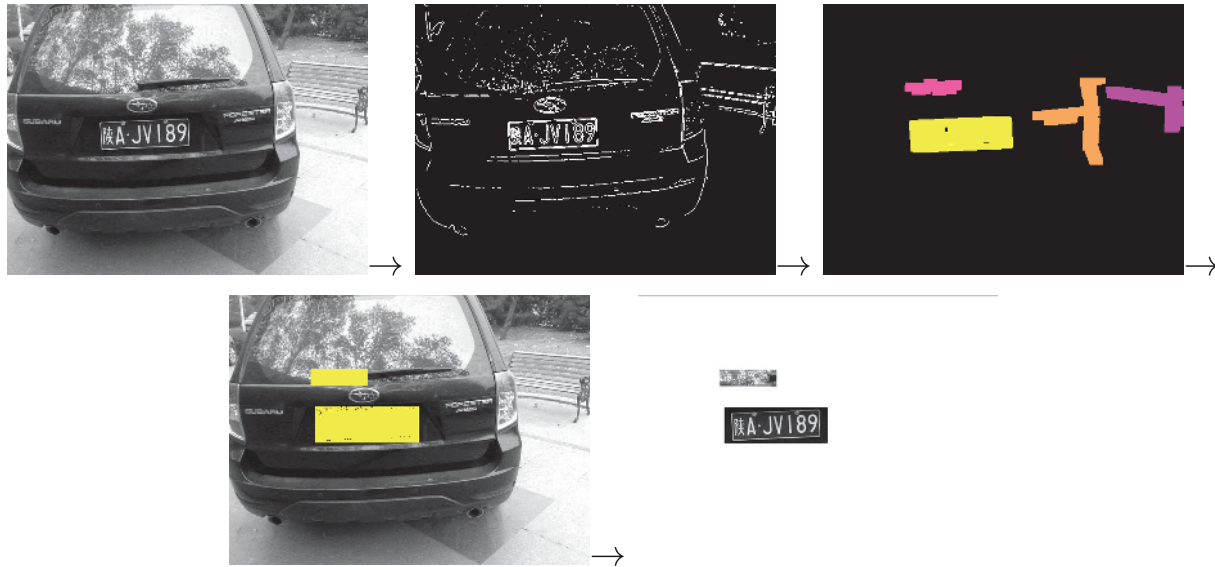
(a) Detection process without the image decomposition step
