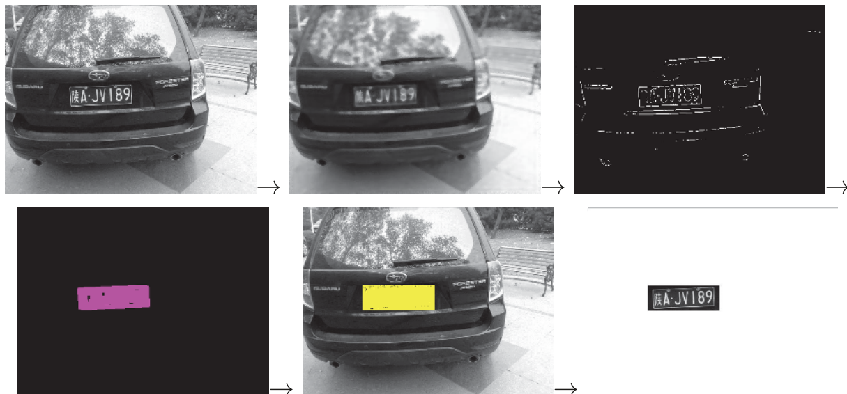
(b) Detection process with the image decomposition step
