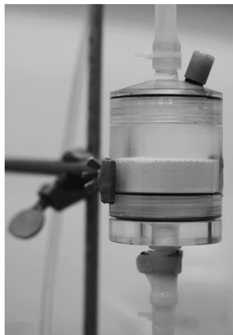
Fig. 1 Column used for concentration of cesium from 100 L of seawater (internal diameter 42 mm, 25 mL of AMP-PAN)
