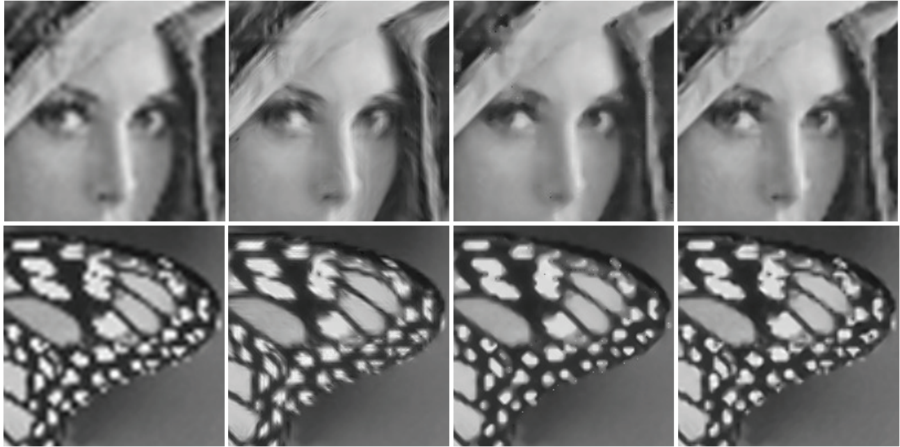
Fig. 6. Results of the Lena and Monarch image at 4 \times interpolation. From left to right: bicubic, NEDI [2], CAI [5] and proposed.
