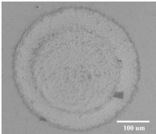
Fig. 2 SEM image of a single-point pattern irradiated at the laser fluence of 0.48 \text{ J/cm}^2 with 100 shots.
