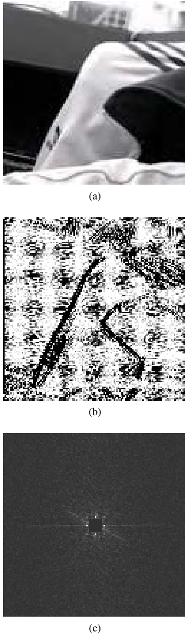
Figure 10. (a) The tampered image; (b) The probability map generated by the Popescu’s method; (c) The frequency response of (b).
