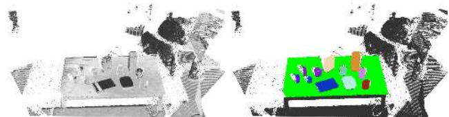
Fig. 8. Left: raw point cloud dataset; right: the segmentation of the table (green) and the objects supported by it (random colors) from the rest of the dataset (black).
