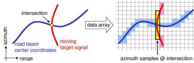
Fig. 1. Principle of the proposed GMTI algorithm. The intersection of the moving vehicle signal with the road corresponds to the vehicle's beam center position.
