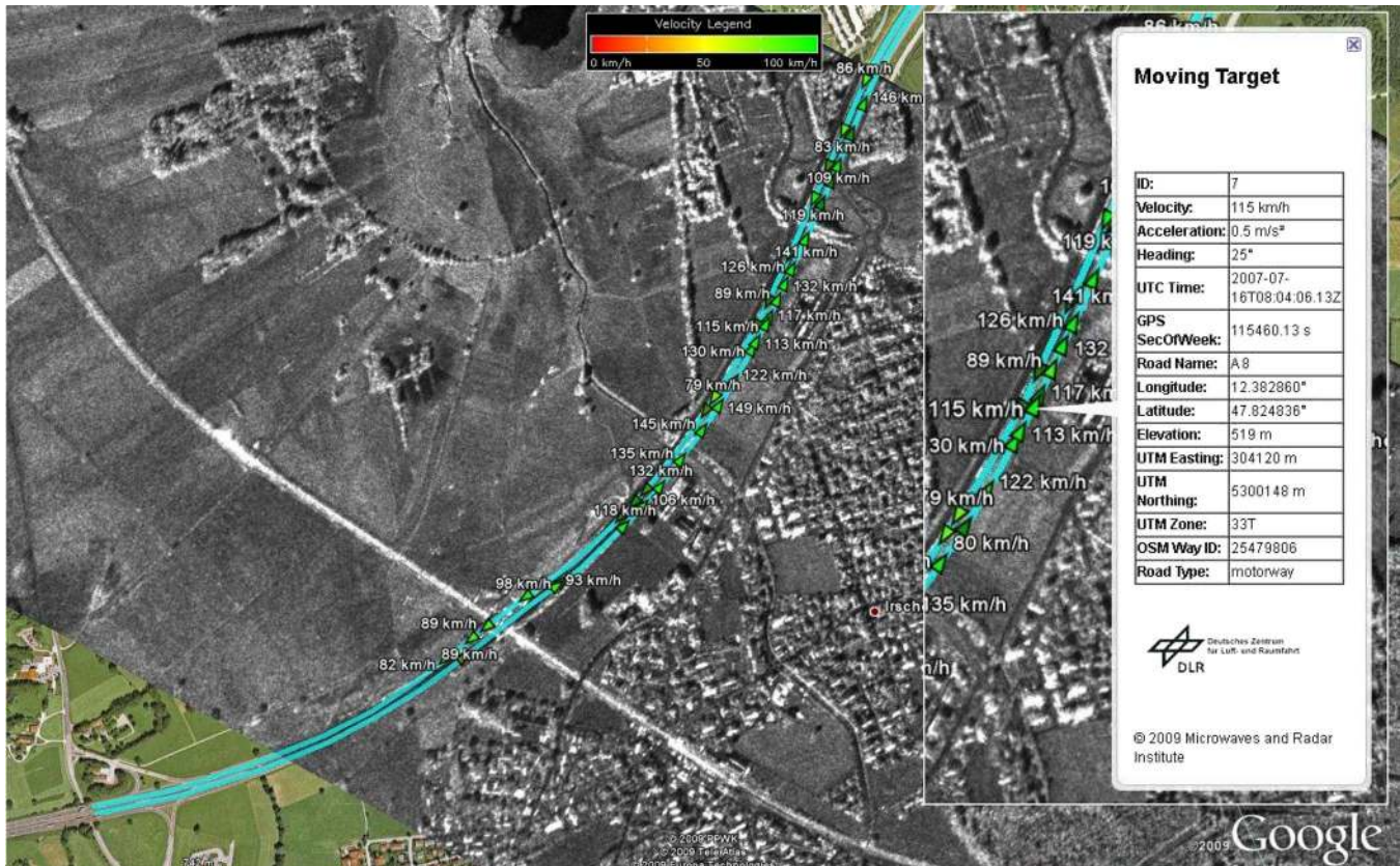
Fig. 21. Google Earth image overlaid with a single-channel SAR image acquired with F-SAR (image not processed with full quality, image size 2.0 \times 2.8 km, data take rc07trmr0302x1). The shown vehicles (color coded triangles) on the autobahn A8 near Chiemsee were automatically detected, and their parameters were automatically estimated using the proposed GMTI algorithm.
