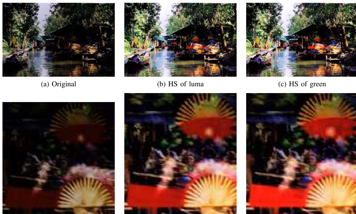
Fig. 3. Top: Original image (a) and enhanced images (b,c) by Alg. IV in this paper with target histogram due to [8] with parameter \mu = 0.9 in (32). The enhancement procedure differs only by the choice of the input histogram. The histogram of the luma, see Remark 2, is used in (b) and the histogram of the green channel only in (c). The result in (c) is surprisingly good. In contrast, replacing the green channel by the red or blue one results in hard defects (not shown here). Bottom: The zoom into the images shows that using the histogram of the green channel introduces some artefacts; the left lower part of image (c) is too red and the upper red fan shows some unpleasant pixels.
