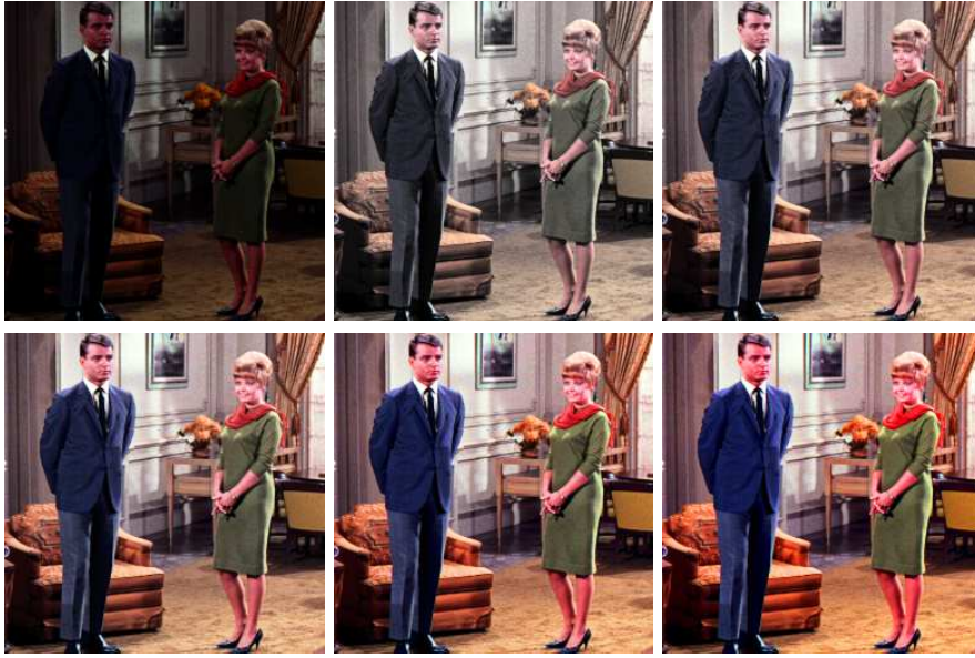
Fig. 5. Enhancement of the image “couple” by our Algorithm III with concave histogram (parameters (l, r) = (0.9, 0.1) ). Original image (top left) and enhancement with \lambda = 0, \frac{1}{4}, \frac{1}{2}, \frac{3}{4}, 1 . The corresponding values \mathcal{U}(\lambda) (in percent of all image pixels) are given by 1.09, 2.20, 3.62, 5.74, 8.70 and the sets \mathcal{L}(\lambda) are empty. A closely similar visual result will be obtained by forming the convex combinations according to (23). While the \hat{w}^\times is very colorful, its additive counterpart \hat{w}^+ appears to be rather gray. All nuances between these images can be obtained by building their convex combinations.
