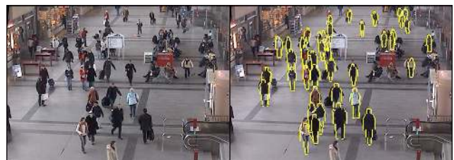
Figure 1. A sample input frame (left) and corresponding detection output generated by the proposed method (right).
