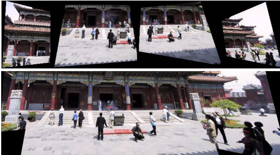
Figure 4: 4 original images from the outdoor panoramic sequence (top) and watershed blending result (down), cropped over the area containing moving people.
