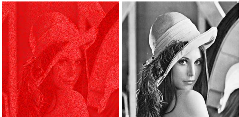
(c) red: inpainting domain D , detected by thresholding (d) inpainted; \epsilon = 5 px, \kappa = 25 , \sigma = 1 px, \rho = 2 px; CPU time: 20 s
