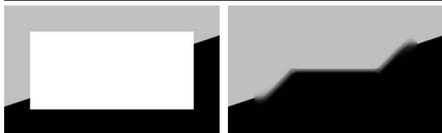
(a) 300 \times 180 \text{ px}^2 ; inpainting domain: 228 \times 108 \text{ px}^2 (b) Telea's method, \epsilon = 6 \text{ px} ; CPU time 0.05 s
