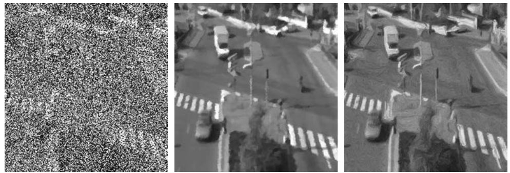
(a) 246 \times 255 \text{ px}^2 (Guichard and Morel [14], Fig. 1.2) (b) Guichard and Morel's [14, Fig. 1.2] result (c) \epsilon = 5 \text{ px}, \kappa = 25, \sigma = 1 \text{ px}, \rho = 2 \text{ px}; CPU: 0.5 s
