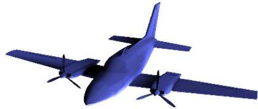
Figure 5: Rendering result of a per vertex light field illumination approach. Although the overall impression of the lighting is plausible, the shadow lacks detail due to insufficient mesh tessellation.
