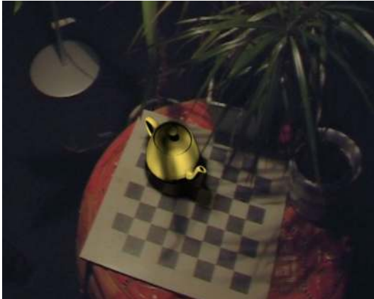
Figure 11: Real world scene with augmented teapot. The shadows of the recorded light field are faithfully rendered on the modeled geometry. Shadows casted by the teapot are generated by the recorded light source and blended with the background image.
