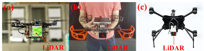
Fig. 6. Three different platforms: (a) 280 mm wheelbase small scale quadrotor UAV carrying a forward-looking Livox Avia LiDAR, (b) handheld platforms, (c) 750 mm wheelbase quadrotor UAV carrying a down-facing Livox Avia LiDAR. All three platforms carry the same DJI Manifold-2C onboard computer. The video of real-world experiments is available at https://youtu.be/20vjGnxszf8 .
