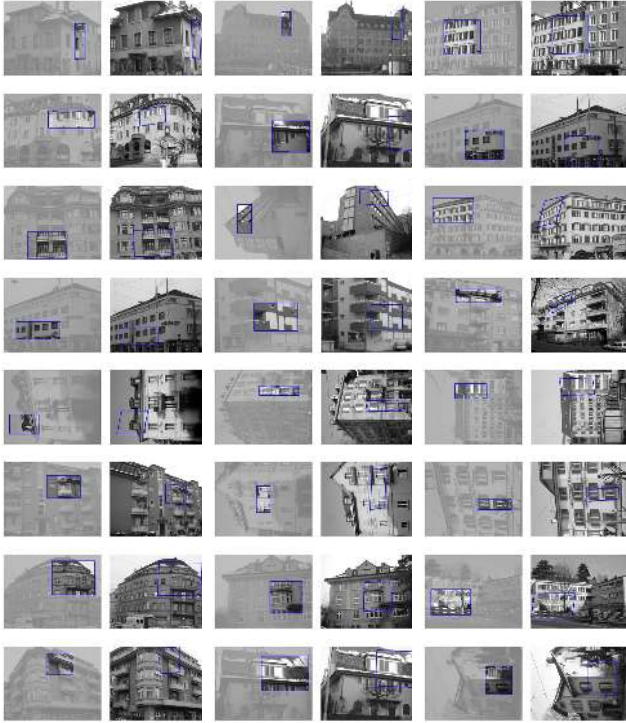
Figure 6. Zurich Dataset [19] - Good Examples: In the blue rectangle on the left of each pair of images is the template presented to Fast-Match. In the blue parallelogram on the right is the region matched by the algorithm. Note that also for some of the non-affine mappings Fast-Match gives a good result.
