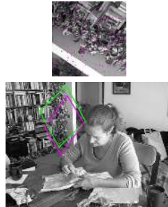
Figure 3. Example from a Fast-Match Run Top: The template (shown enlarged for clarity), with the 152 pixels that Fast-Match samples. Bottom: Target image, with origin of the template (ground truth location) in green and a candidate area it is mapped to in magenta.
