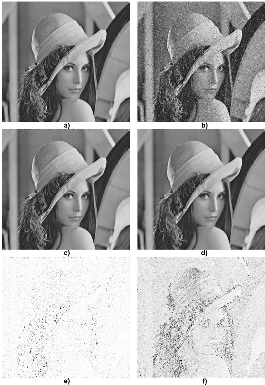
Fig. 4. Noise reduction effect of the proposed filter as compared with the standard VMF: a) colour test image LENA , b) image distorted by 4 % impulsive noise, c) new method ( 3 \times 3 window, \beta = 0.5 ), d) VMF, e) and f) the absolute difference between the original and filtered image (the RGB values were multiplied by factor 10).
