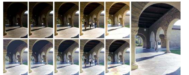
Fig. 3. Median image generation with histogram equalization and median filtering. Top-left: the original "Arch" LDR image sequence. Bottom-left: the histogram equalized "Arch" LDR sequence. Right: the median image of histogram equalized LDR image sequence.
