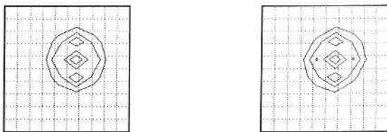
Figure 7 : The corresponding power spectra of the two PET images shown in Figure 6, illustrating the detrimental influence of the rectangular image frame on rotation.
