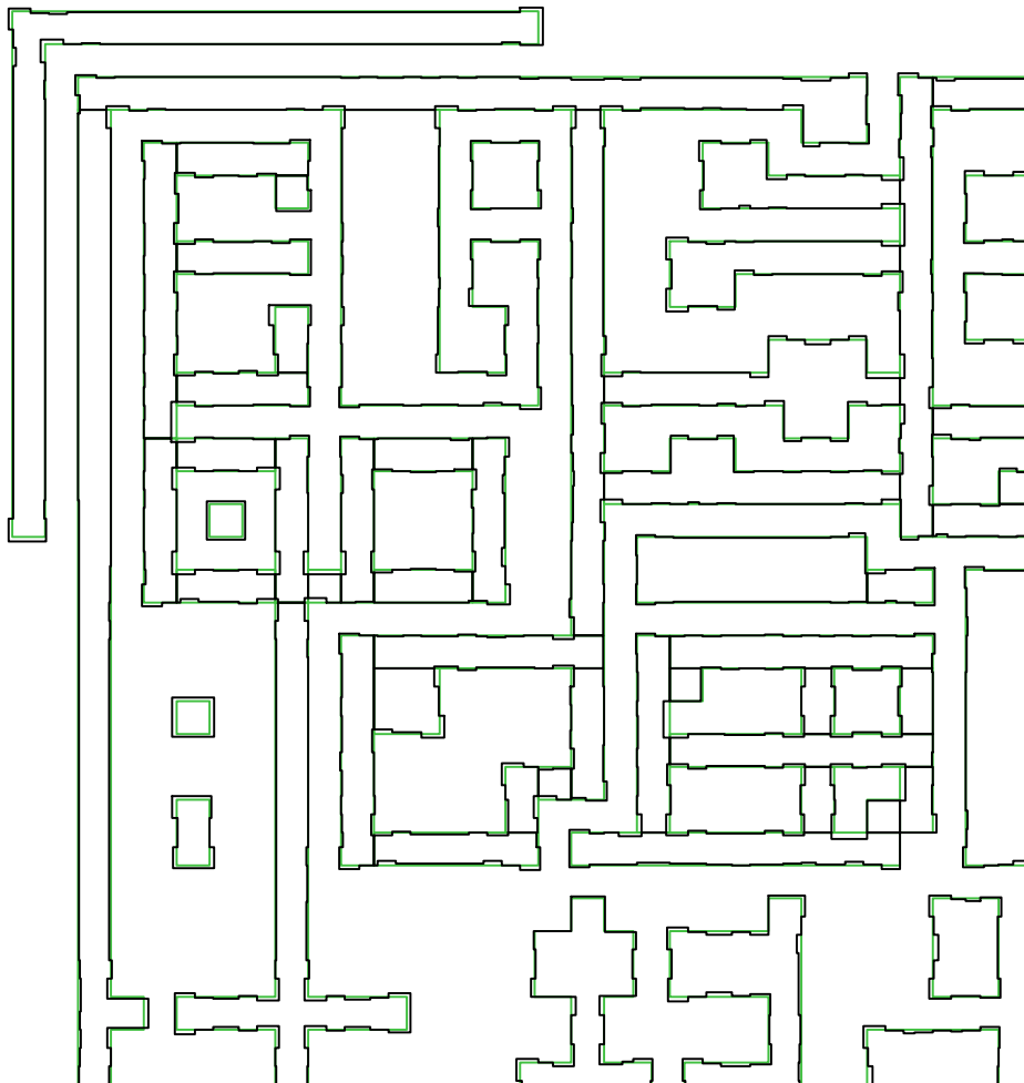
Figure 2.15: OPC correction of a 0.36 \mu\text{m} pattern
