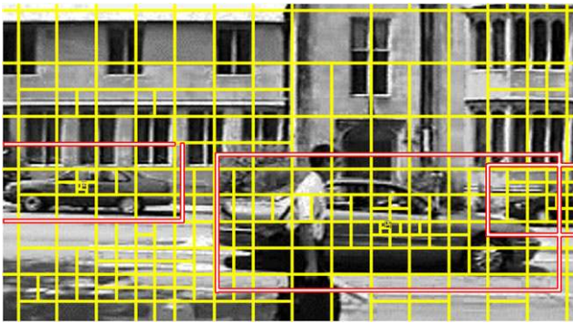
Fig. 9 (Color online) Adaptive subdivision of the search space. The object center serves as hypothesis parametrisation. Each yellow box corresponds to a set of hypotheses (which comprises objects whose center is within the box). The discretisation around object centers is much finer than on background regions
