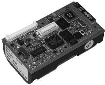
Figure 1. The BTnode rev3 uses a four layer PCB with all components mounted on the top and a 2xAA battery case underneath.
