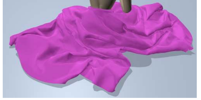
Figure 7: Cloth simulation: The cloth is modeled using 12.5K triangles. Our proximity computation algorithm is able to perform the N-body distance query at object-space precision within 400 – 600 ms.
