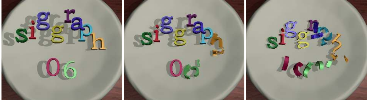
Figure 1: Multiple deformable models simulation: This sequence shows the positions of the objects at three time instances in a simulation. The environment initially consists of 10 deforming objects represented using 5.5K triangles. As the simulation proceeds, the objects break into 25 sub-objects. Our algorithm is able to perform collision and separation distance computations, including self-collisions, among dynamically generated objects within 120 ms on a high-end PC.
