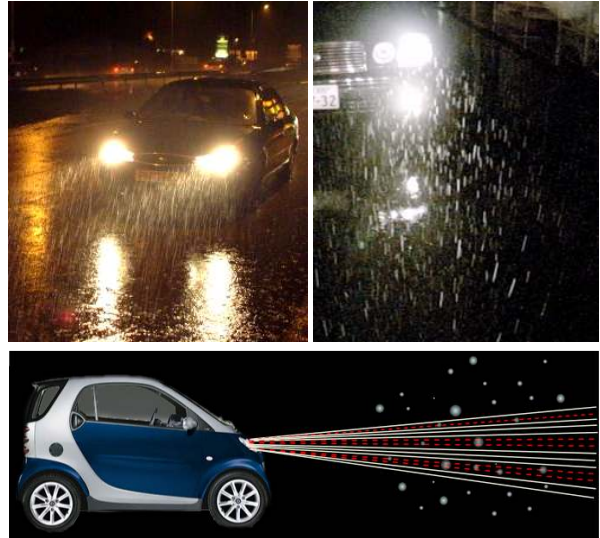
Figure 1. At night, illuminated rain or snow appears as a bright flickering (distracting) pattern that reduces driver visibility (top). We propose a reactive system (bottom) that deactivates only those light rays that intersect particles such as raindrops, snowflakes, and hailstones diminishing the visual effect of precipitation.
