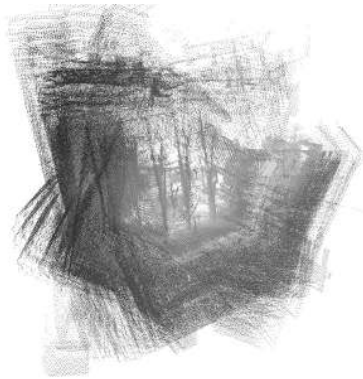
(f) The top view of the odometry based point-cloud map. The robot starts at upper right.
