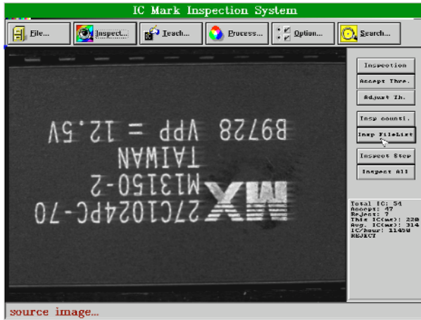
Fig. 14. The defective IC print mark with partial bad contrast.
