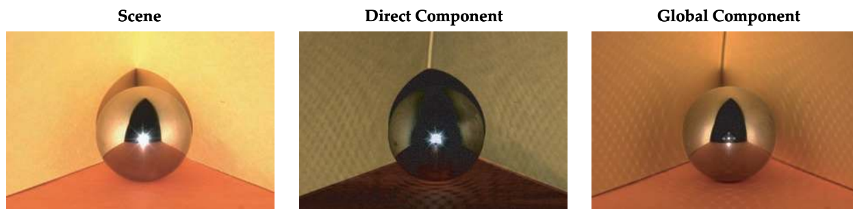
Figure 8: Separation results using checkerboard illumination shifts for a scene that includes a mirror sphere and three diffuse walls around it. The separation method fails in this case as the scene violates our assumption that the global function at each point is smooth compared to the illumination frequency. As a result, we see checker-like artifacts in the measured direct and global images.
