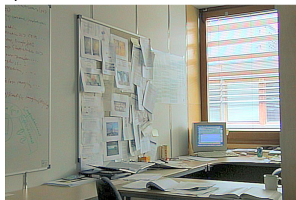
Figure 2 , Result of low dynamic range display mapped from a HDR radiance map with a dynamic range of 602,055 : 1, \alpha = 0.5
