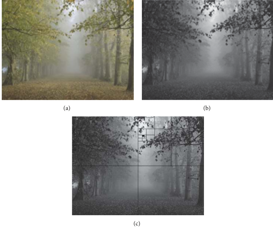
FIGURE 1: Illustration of quad-tree algorithm. (a) Original image. (b) Channel minimum map. (c) Result of quad-tree division.
