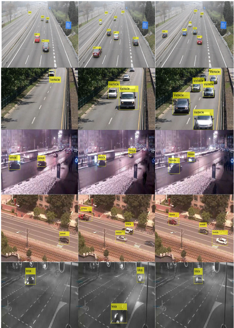
Fig. 8 Sample detection results using experiment III. Top row: crowded and Cloudy. Second and fourth row: different camera view, sunny day, and waving trees. Third and Bottom row: Night scenes with changed light
