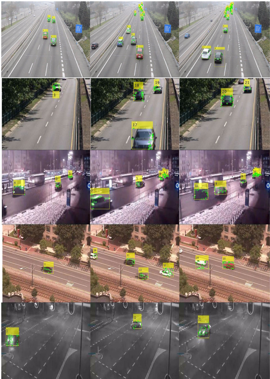
Fig. 9 Sample counting results using experiment III. Top row: crowded and Cloudy. Second and fourth row: different camera view, sunny day, and waving trees. Third and Bottom row: Night scenes with changed light
