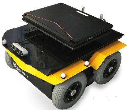
Fig. 34: Ground robot used in the experiments. It is equipped with an Intel ® RealSense Depth Camera D435, and an i7-7700HQ laptop.
