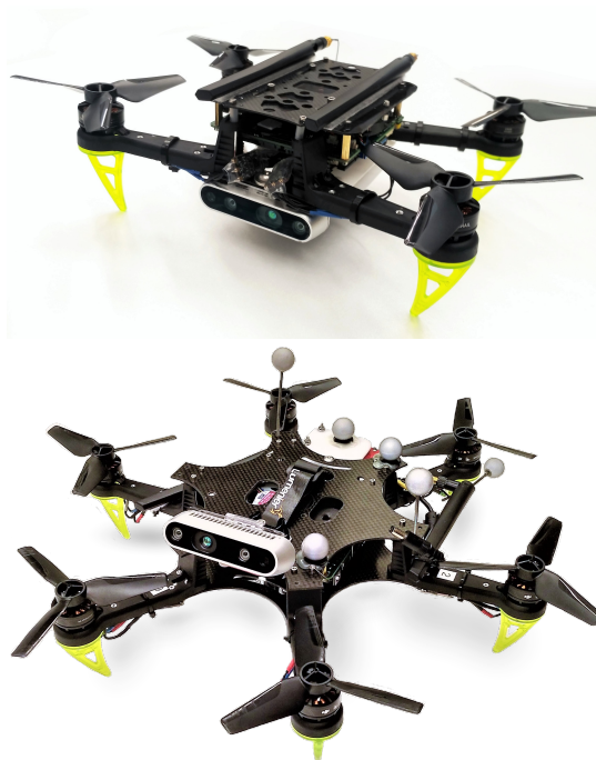
Fig. 23: Quadrotor (top) used in the experiments 1-4 and hexarotor (bottom) used in the experiments 5 and 6. Both are equipped with a Qualcomm® SnapDragon Flight, an Intel® NUC i7DNK, and an Intel® RealSense Depth Camera D435.
