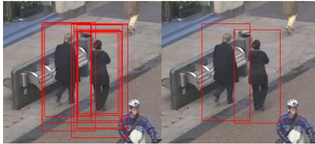
Figure 9: Non-maximal suppression. left - all detections, right - fused detections
