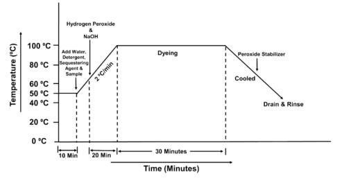
Figure 1 Process curve of scouring and bleaching in same bath
