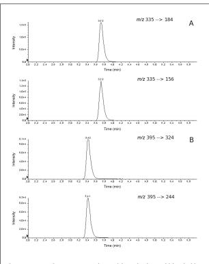
Figure 2. MRM chromatograms obtained from the femoral blood (dilution 1:10) containing strychnine (internal standard) (A) and  $1.5 \mu$ g/mL brucine (B).
