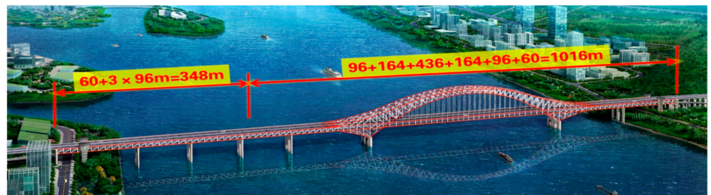
Figure 2. General layout of Guangzhou Mingzhu Bay Bridge.
