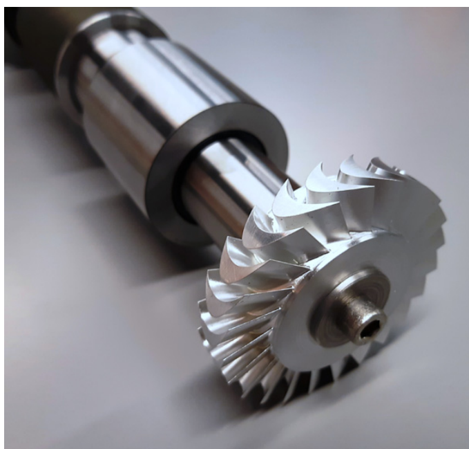
Figure 4. Photograph of the real rotor with the turbine disc that was subjected to analysis.
