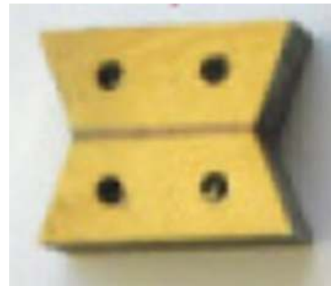
FIGURE 2: Adhesive butterfly joint.
