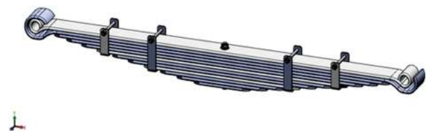
FIGURE 10: CAD model of the leaf springs.
