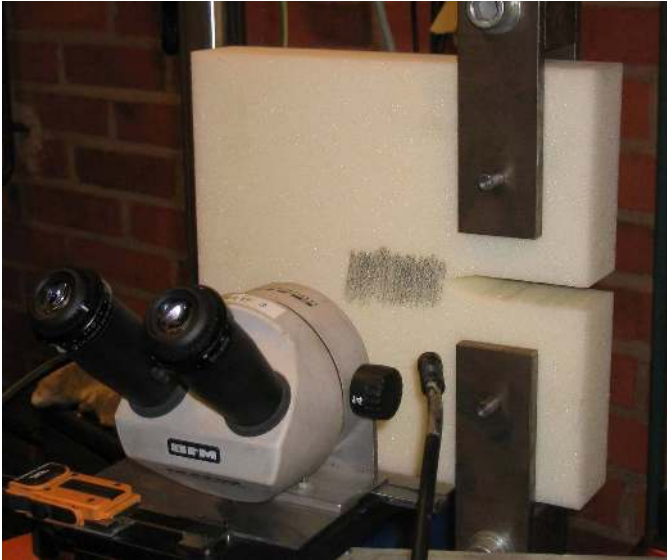
Figure 3 Geometry and photograph of the CT specimen
