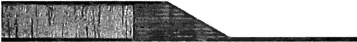
Figure 194. Detail of Fillet Region Showing Solid DB400 Laminate Fillet.
