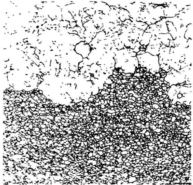
Fig. 3.38 Photomicrograph showing the pretest structure of the 348 stainless steel (longitudinal cross section) used in low-cycle-fatigue testing ( 50\text{HNO}_3 , 50\text{H}_2\text{O} , electrolytic etch; magnification, 100\times ).
