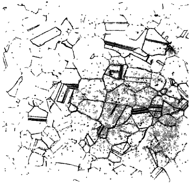
Fig. 3.39 Photomicrograph showing the pretest structure of the 316 stainless steel (longitudinal cross section) used in low-cycle-fatigue testing [ 22\text{H}_2\text{SO}_4 , 12\text{H}_2\text{O}_2 (30%), 66\text{H}_2\text{O} , electrolytic etch; magnification, 100\times ].
