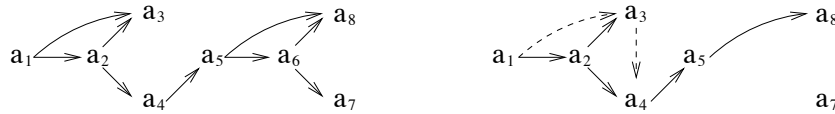
Figure 1. (left) A causality graph. On this example, a_2 is a consequence of a_1 , a_5 is causally related to a_2 (and thus to a_1 ), a_3 and a_4 are concurrent. (right) Structure of observations: a damaged or “incomplete” causality graph. The loss of a_6 cancels some causal links. Other relations can’t be observed (dashed arrows): these arrows can either be present or absent.
