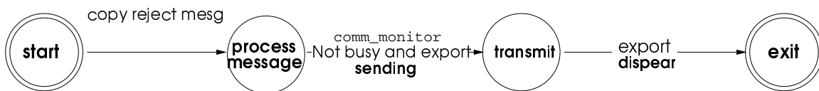
Figure A.27: Coordination layer communication rejection automata
