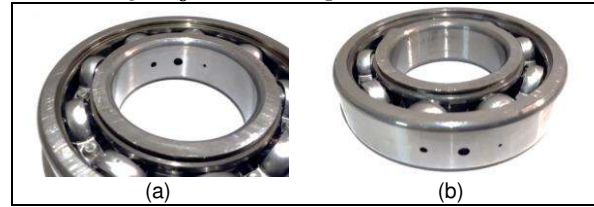
Fig. 6. Examples of multiple defects introduced to the bearings. (a) Defects on inner raceway. (b) Defects on outer raceway.
