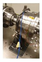
Figure 3. Placement and direction of installation of accelerometers.
