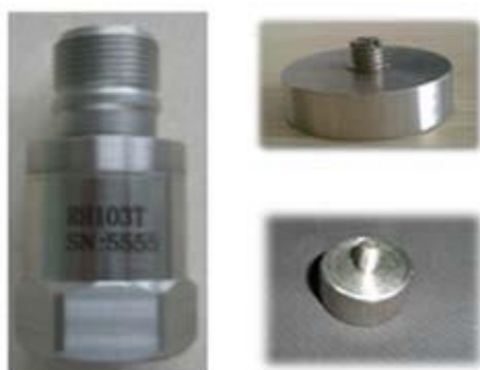
Figure 2. Photos of a vibration sensor and its base used in the main chain of the wind turbine.
