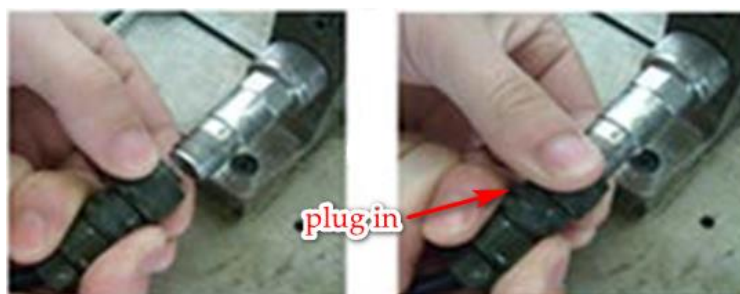
Figure 3. Method to equip the vibrating sensor.
