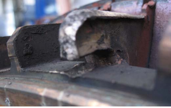
Fig. 17. Broken bar of the 3.15 MW motor used for the experimental validation of the proposed method.
