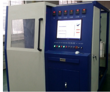
Fig.4.a) Hydraulic Pump Full Life Test Platform.
