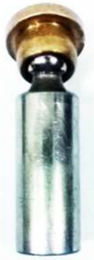
Fig.5.b) Piston failure of loose slipper.
