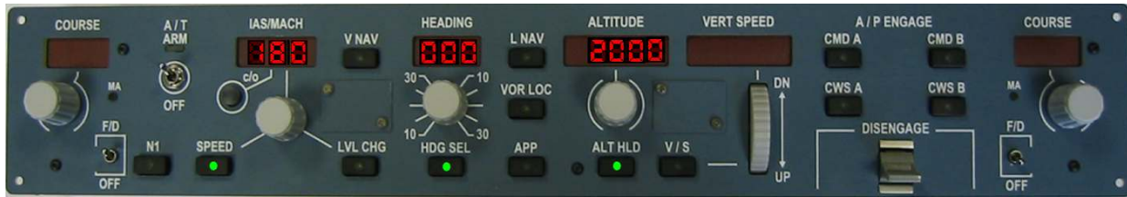
Fig. 3. Mode control panel (MCP)
