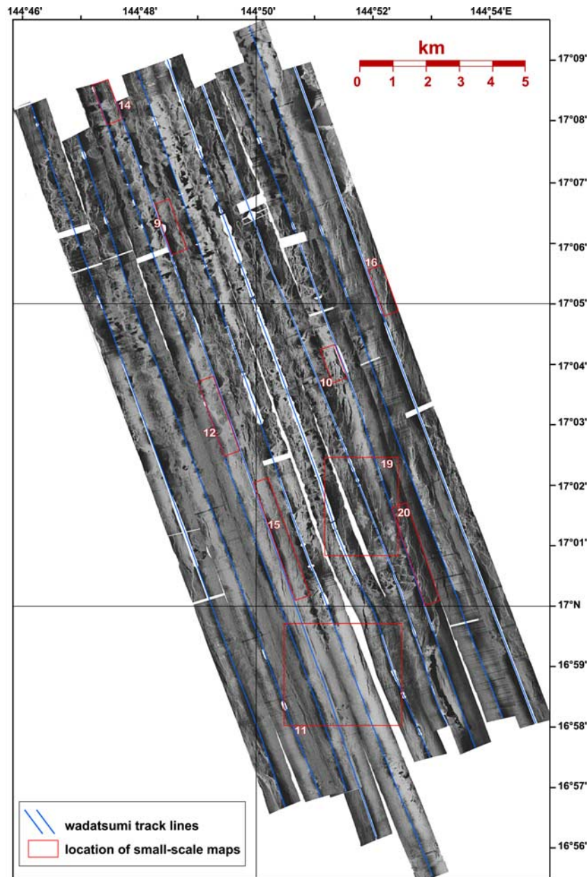
Figure 7. Side-scan mosaic of the area surveyed by Wadatsumi. Bright is reflective seafloor indicative of recent volcanic products and fault scarps facing toward the instrument. Dark is low backscatter seafloor, indicative of old volcanic constructions, sedimented areas, shadows, and scarps facing away from the instrument. Frames numbered 9 to 20 are locations of Wadatsumi small-scale mosaics shown in figures of the same number.
